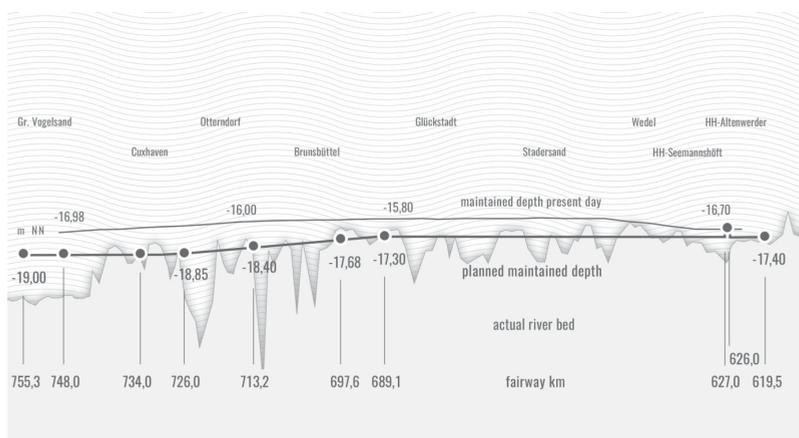
Figure 1. Current state and planned adjustment of the navigation channel
