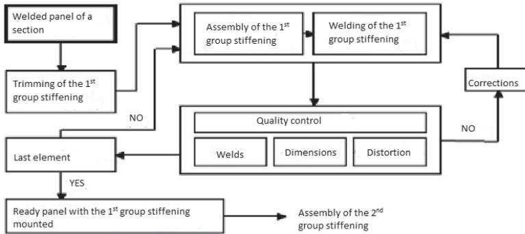
Figure 2. The second stage of the construction of a section for an offshore vessel
