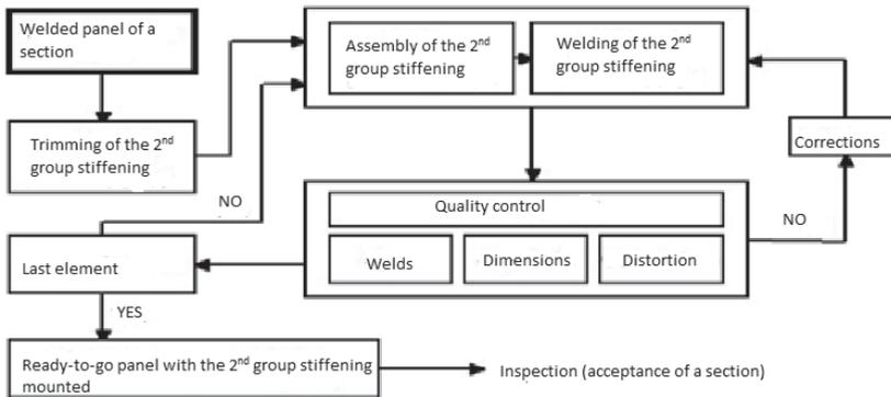
Figure 3. The third stage of the construction of a section for an offshore vessel
