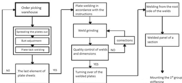
Figure 1. The first stage of the construction of a section for an offshore vessel
